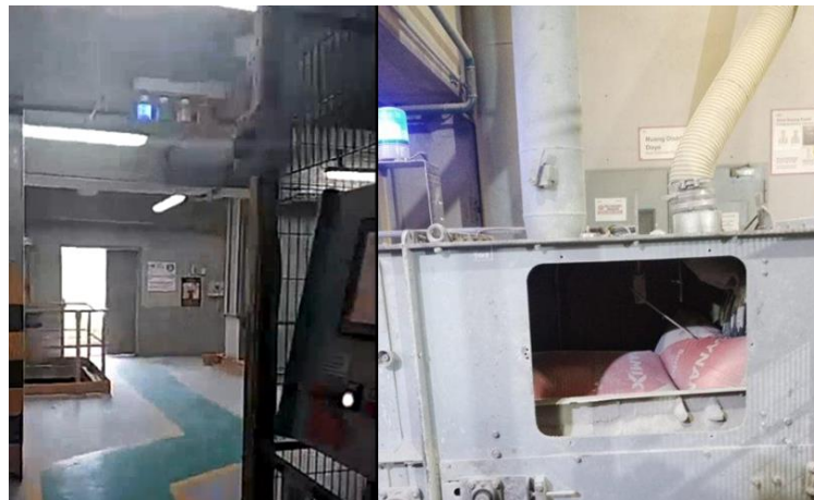
Figure 3 Installation Of Blocking Indication Sensor Lamp
